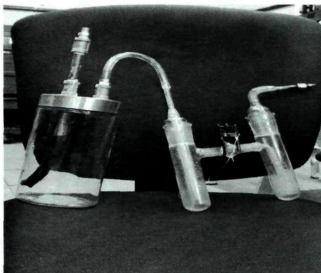
Figure A.1 Condensation system
