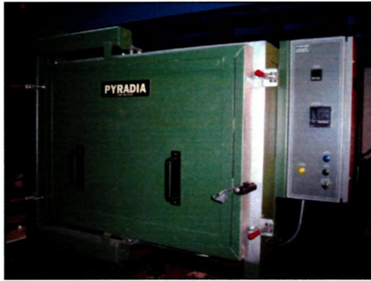
Figure 3.2 Forced-air electric furnace.
