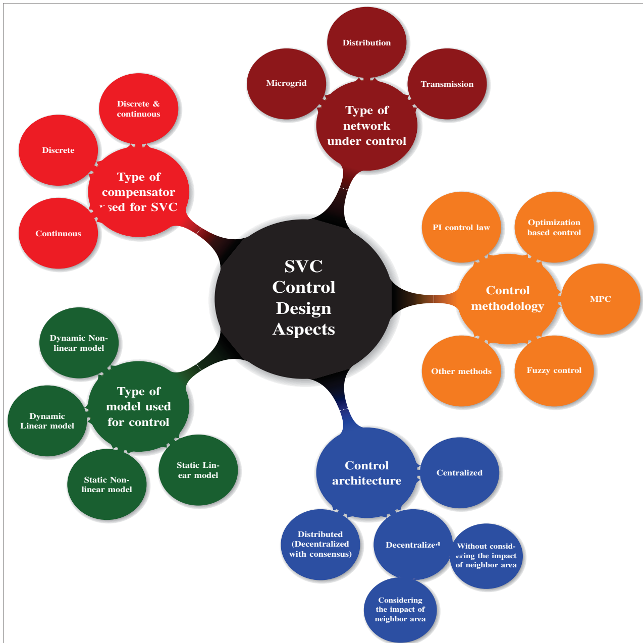
Figure 2.1 Classification of SVC Control desing aspects
