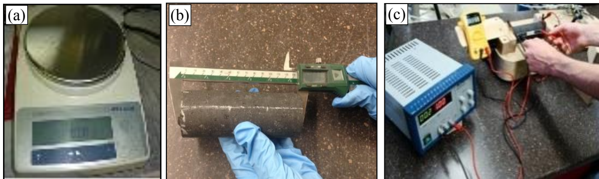
Figure 3.11: Density and resistivity measurements of cylindrical anode samples: (a) Balance, (b) Slide caliper, (c) Set-up for the electrical resistivity measurement of anode samples at UQAC.
